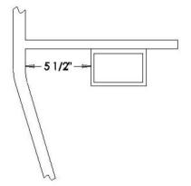
Note: The measurement for the battery box offset will be taken at the point closest to the crossmember, from the inside of the framerail to the otside of the battery box. Engine Type: Air cooled 4-Stroke gasoline
